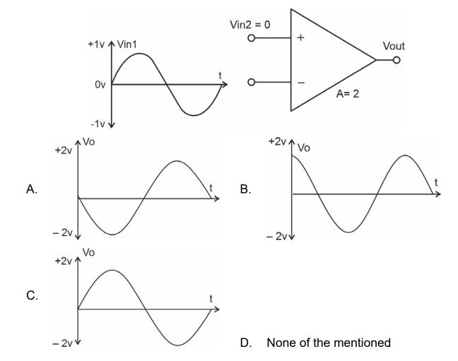
19. Determine the output voltage from the following circuit diagram?
